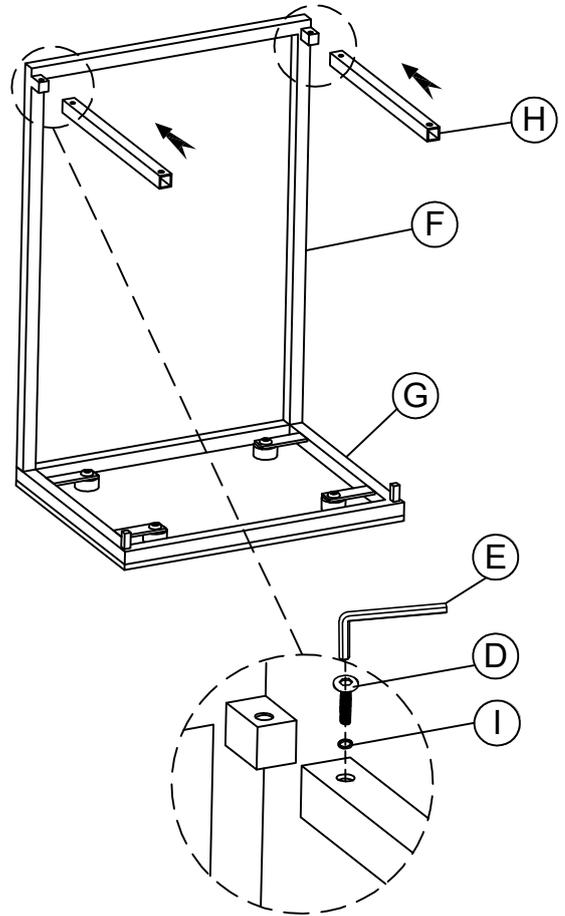
Step 6: Using the Allen key to tighten all bolts.
