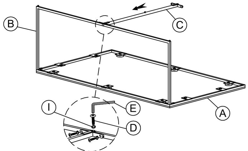
Step 3: Using the Allen key to tighten all bolts.
