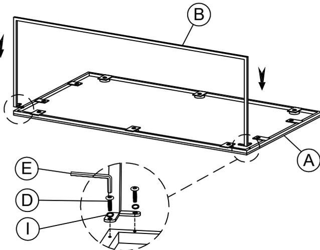
Step 2: Do not fully tighten the bolts
